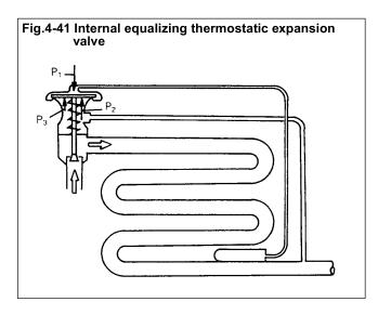
Thermostatic expansion valve has been substituted by electronic expansion valve in recent years, resulting in few models using it. In order to differentiate the valve in the piping circuit diagram, probing the presence of the feeler bulb as shown in the figure on the right locates the thermostatic expansion valve. (See Fig. 4-42)
