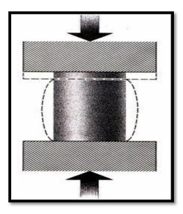
Figure 2. Compression test of ductile material.
