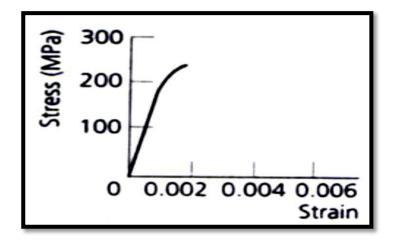
Figure 4. Typical stress-strain curve of grey cast iron (Brittle Material).
