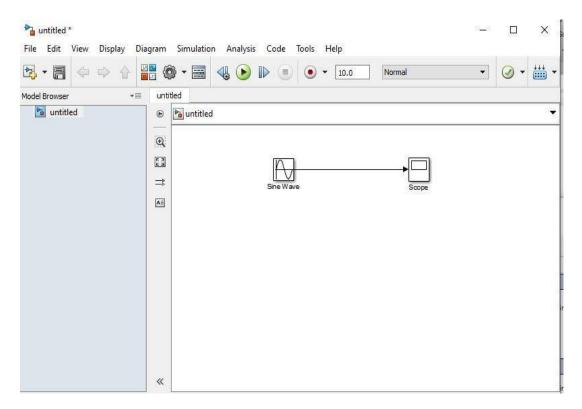
Run the simulation and double click on the scope to see the results.
