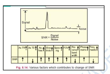
Fig. (9) : Various factors which contributes to change of SNR
