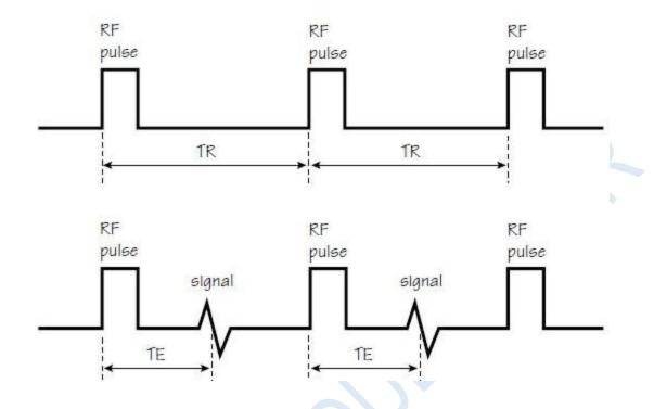
Fig.(2): A basic pulse sequence.
