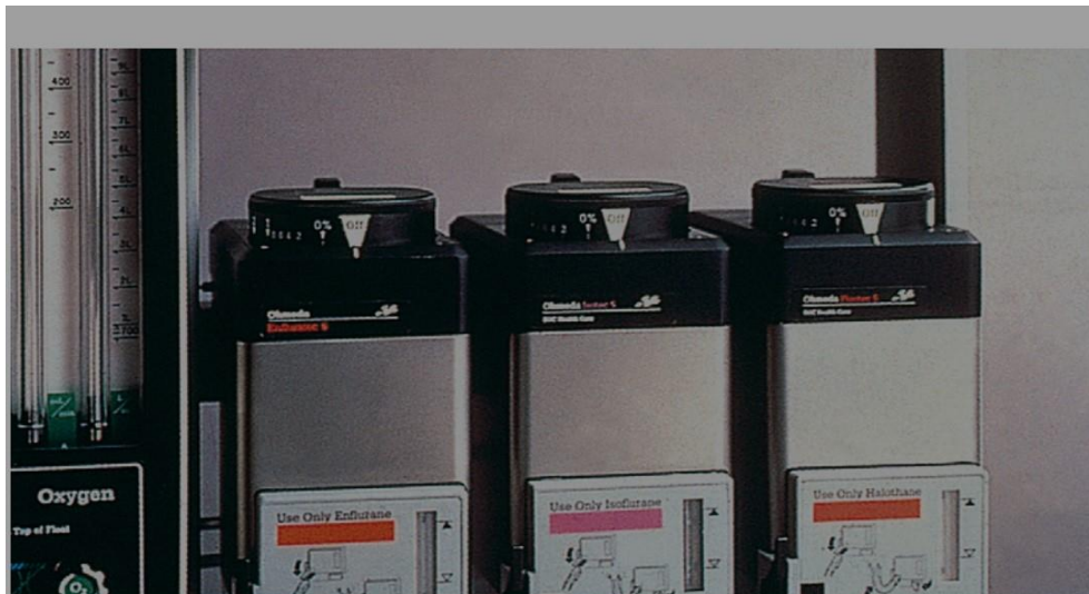
Fig. 2.17 Tec Mk 5 vaporizers mounted on the back bar of an anaesthetic machine.
