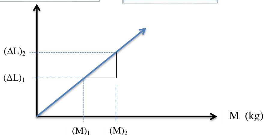
$$\text{Slope} = \frac{\Delta(\Delta L)}{\Delta(M)}, = \frac{\Delta L_2 - \Delta L_1}{M_2 - M_1}$$
