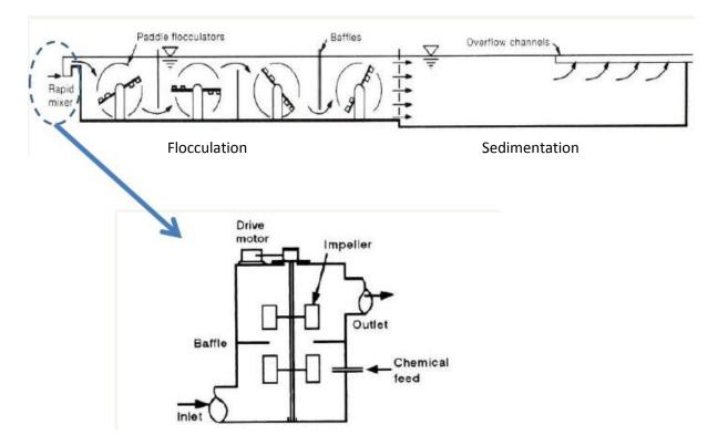
**Coagulation** is the destabilization of colloids by addition of chemicals that neutralize the negative charges.
