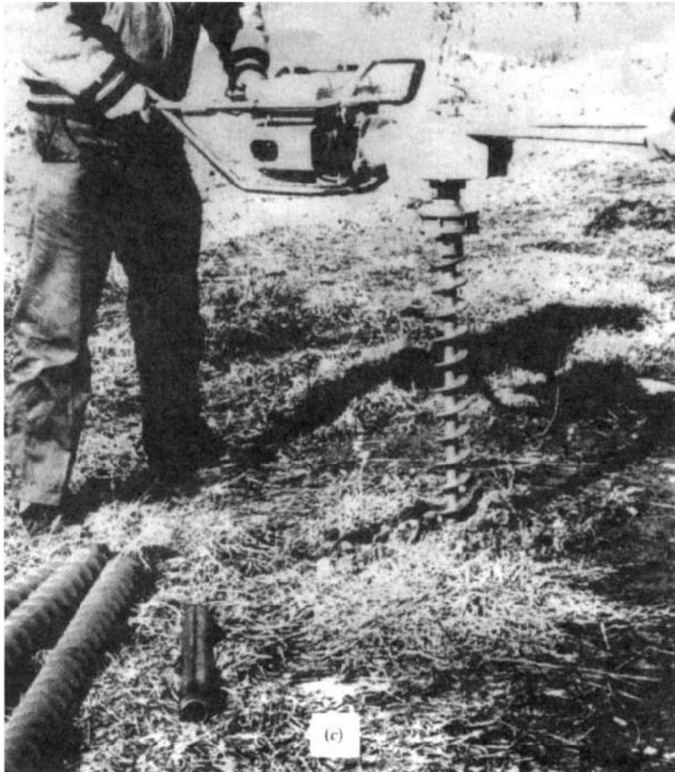
Figure 3-1 Hand tools for soil exploration. (a), (b) Hand augers; (c) gasoline-engine-powered hand auger with additional auger flights in the foreground together with hand-driven sample tube.
