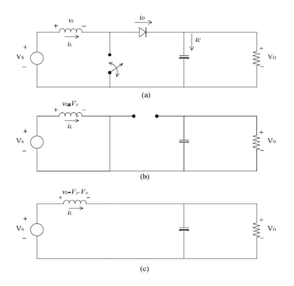
Figure: The boost converter: (a) Circuit. (b) Equivalent for the switch closed. (c) Equivalent for the switch open.
