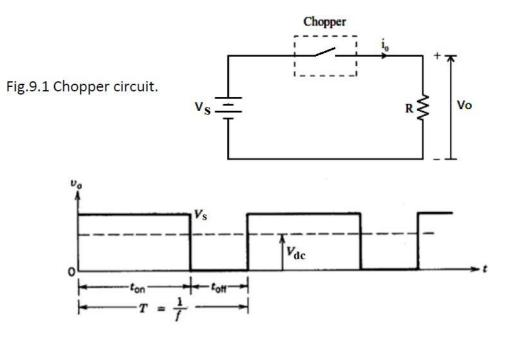
Fig.9.2 Chopper output voltage waveform, R- load.
