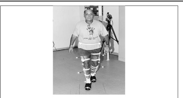
**Figure 3:** This individual is wearing reflective spheres. An infrared camera system can track limb segment motion as the patient walks across the field of view.
