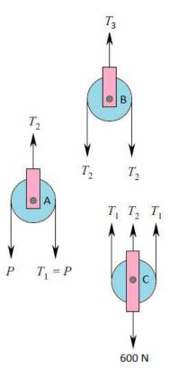
**Example No. 3:** For the system of pulleys shown in Figure, determine the value of W so that the system to maintain equilibrium if value of P is 50 N. Neglect friction and the weights of the pulleys.
