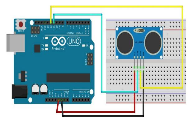
The Ground and the VCC pins of the module needs to be connected to the Ground and the 5 volts pins on the Arduino Board respectively and the trig and echo pins to any Digital I/O pin on the Arduino Board.
