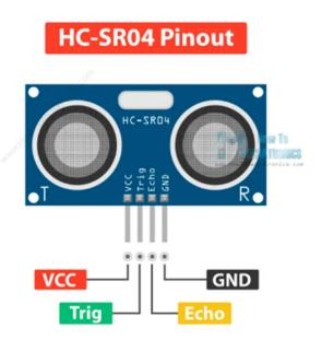
The sensor has 4 pins. *VCC* and *GND* go to *5V* and *GND* pins on the Arduino, and the *Trig* and *Echo* go to any digital Arduino pin. Using the *Trig* pin we send the ultrasound wave from the transmitter, and with the *Echo* pin we listen for the reflected signal.
