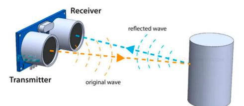
In order to generate the ultrasound we need to set the Trig pin on a High State for 10  $\mu$ s. That will send out an 8 cycle ultrasonic burst which will travel at the **speed of sound**. The Echo pins goes high right away after that 8 cycle ultrasonic burst is sent, and it starts listening or waiting for that wave to be reflected from an object. For that purpose we are using the following basic formula for calculating distance:
