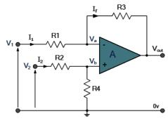
When resistors, R1 = R2 and R3 = R4 the above transfer function for the differential amplifier can be simplified to the following expression:
