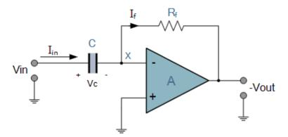
At low frequencies the reactance of the capacitor is "High" resulting in a low gain (Rf/Xc) and low output voltage from the op-amp. At higher frequencies the reactance of the capacitor is much lower resulting in a higher gain and higher output voltage from the differentiator amplifier.
