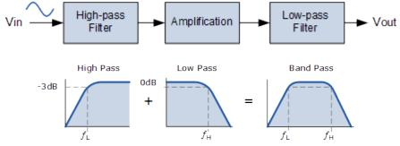
The cut-off or corner frequency of the low pass filter (LPF) is higher than the cut-off frequency of the high pass filter (HPF) and the difference between the frequencies at the -3dB point will determine the "bandwidth" of the band pass filter while attenuating any signals outside of these points. One way of making a very simple Active Band Pass Filter is to connect the basic passive high and low pass filters we look at previously to an amplifying op-amp circuit as shown:
