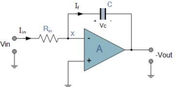
The **Op-amp Integrator** is an operational amplifier circuit that performs the mathematical operation of **Integration**, where the output to respond to changes in the input voltage over time as the op-amp integrator produces an *output voltage which is proportional to the integral of the input voltage*.
