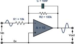
At low frequencies the capacitors reactance is much higher than R2, so the dc gain is set by the standard inverting formula of: -R2/R1 = 10, for this example. As the frequency increases the capacitors reactance decreases reducing the impedance of the parallel combination of Xc||R2, until eventually at a high enough frequency, Xc reduces to zero.
