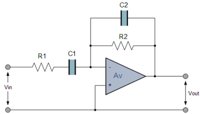
$$\text{Voltage Gain} = -\frac{R_2}{R_1}, \quad f_{c_1} = \frac{1}{2\pi R_1 C_1}, \quad f_{c_2} = \frac{1}{2\pi R_2 C_2}$$
