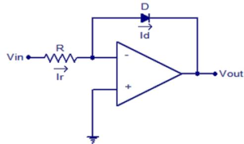
Anti-log amplifier is one which provides output proportional to the anti-log, i.e. exponential to the input voltage. If  $V_{in}$  is the input signal applied to an Anti-log amplifier then the output is  $V_{out} = K \exp(a \cdot V_{in})$  where  $K$  is proportionality constant,  $a$  is constant.
