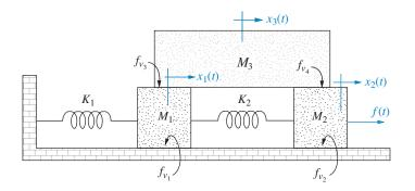
FIGURE 2.20 Three-degreesof-freedom translational mechanical system
