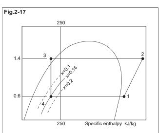
Note: It is understood that, even though the refrigerant is in the lowtemperature low- pressure liquid state when it is discharged from the expansion valve, actually moist vapor having a dryness factor of 0.16 enters the evaporator.
