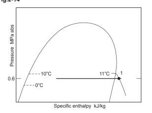
Note: Strictly speaking, the pressure varies while showing a slight drop in the evaporation process, while the pressure is assumed to be constant on the P-h Chart.
