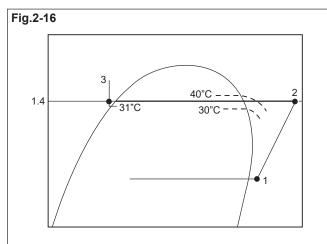
Note: The pressure also varies while showing a slight drop in the condensation process, while the pressure is assumed to be constant on the P-h Chart.
