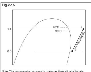
Note: The compression process is drawn as theoretical adiabatic compression. Therefore, it may be slightly different from that in actual operation.
