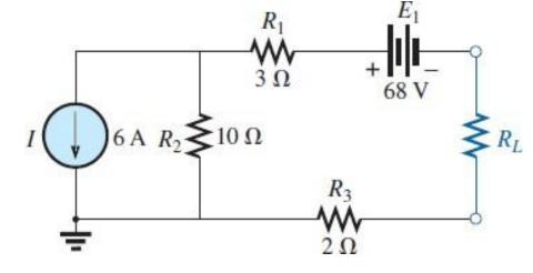
$R_{Th} = R_1 + R_2 + R_3 = 3 \Omega + 10 \Omega + 2 \Omega = 15 \Omega$  $-V_1 = 0V +$  $E_1$  $R_L = R_{Th} = 15 \ \Omega$  $V_1 = V_3 = 0 V$  $R_1 = 3 \Omega$ 68 V I = $V_2 \ge R_2 = 10 \Omega$  $E_{Th}$  $V_2 = I_2 R_2 = I R_2 = (6 \text{ A})(10 \Omega) = 60 \text{ V}$  $E_{Th} = V_2 + E = 60 \text{ V} + 68 \text{ V} = 128 \text{ V}$ 6 A I = 6 A6 A  $P_{L_{\text{max}}} = \frac{E_{Th}^2}{4R_{Th}} = \frac{(128 \text{ V})^2}{4(15 \Omega)} = 273.07 \text{ W}$  $R_3 = 2 \Omega$  $+ V_3 = 0 V -$
