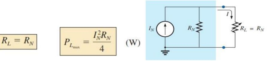
Consider the circuit in Fig. where the load resistance is set at 100  $\Omega$  and the power to the Thévenin resistance and to the load are calculated as follows:
