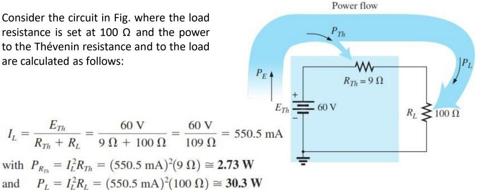
The results clearly show that most of the power supplied by the battery is getting to the load—a desirable attribute on an efficiency basis. However, the power getting to the load is only 30.3 W compared to the 100 W obtained under maximum power conditions.
