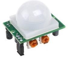
The sensor in the figure above has two built-in potentiometers to adjust the delay time (the potentiometer at the left) and the sensitivity (the potentiometer at the right).
