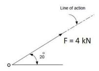
**Forces:** is the action of one body on another which changes or tends to change the motion of the body acted on. The action of a force is characterized by:
