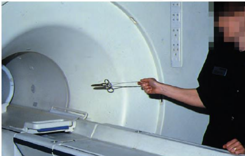
Figure 55.1 The pulling power of a pair of scissors in a 1.5 T system.
