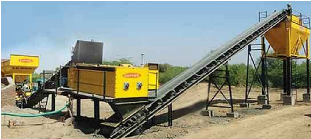
Fig.2 Wet Mix Macadam Plant
