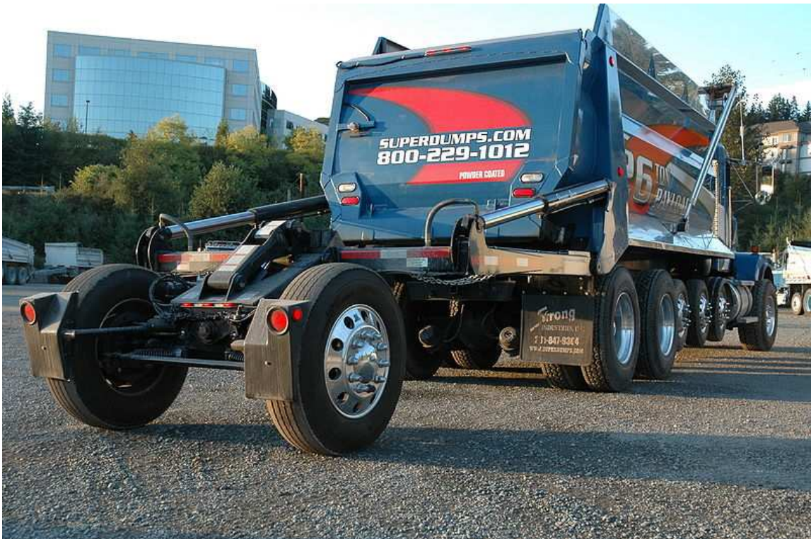
Fig.6 Super dump body and trailing axle
