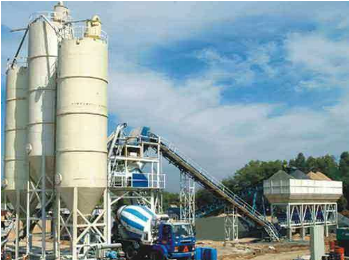
Fig. 1 Horizontal concrete batching and mixing plant
