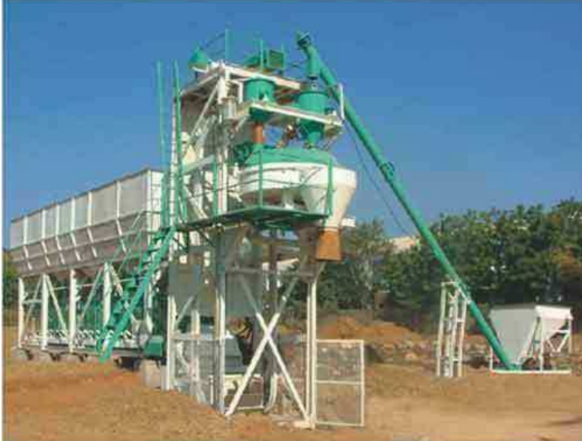
Fig. 3 Compact Concrete Batching/Mixing Plant. (Inline Bin)
