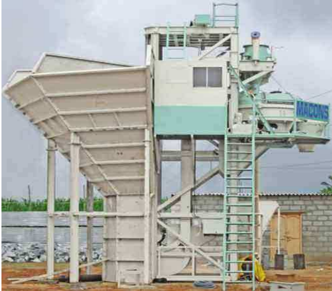
Fig. 4 Compact Concrete Batching/Mixing Plant(Pocket Type)
