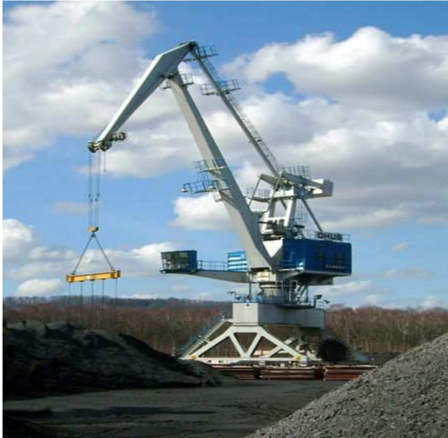
Fig.8 Level Luffing crane
