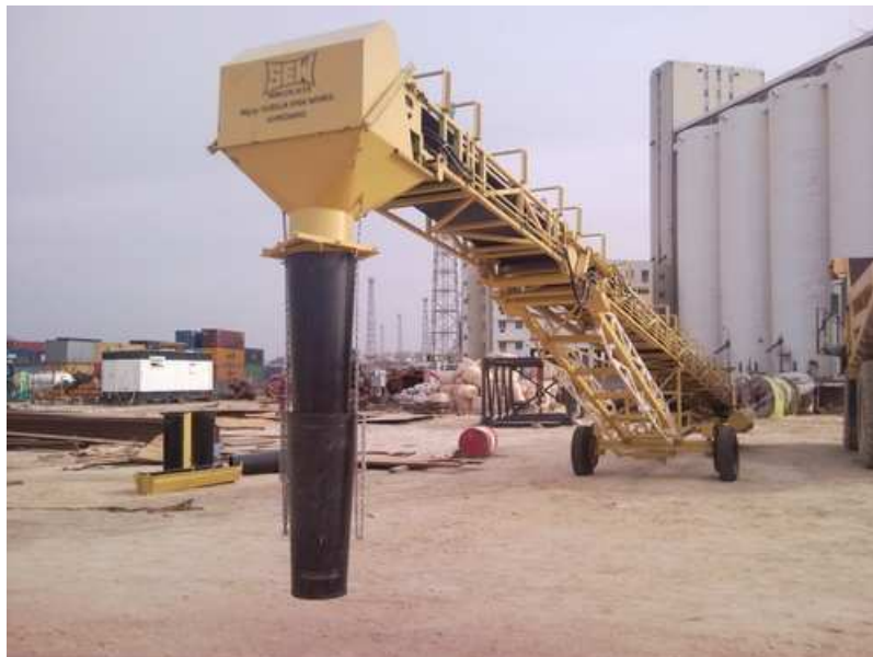
Fig. 7(i) Mobile Concrete Placer-56/650
