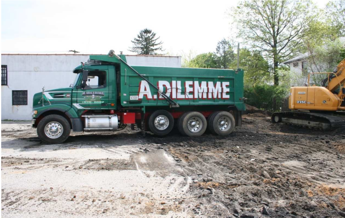
Fig.2 Another kind of 8x4 dump truck: three rear axles (two powered, one lift)
