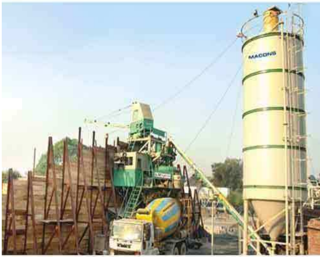
Fig. 2 Compact Concrete Batching/Mixing Plant (Scrapper Type)
