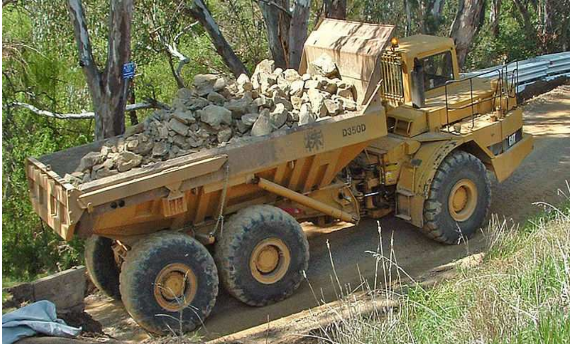
Fig.3 Articulated dump truck or dumper
