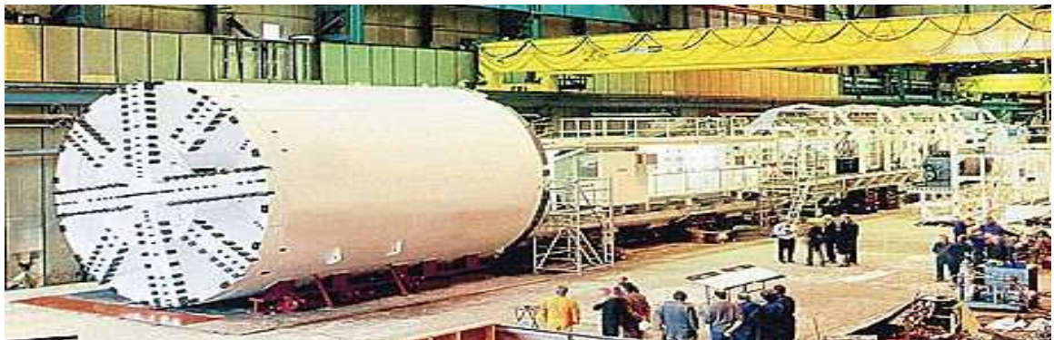
Fig. 7 Slurry Pressure Balance Tunnel Boring Machine
