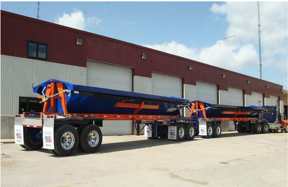
Fig.9 Side Dump Truck
