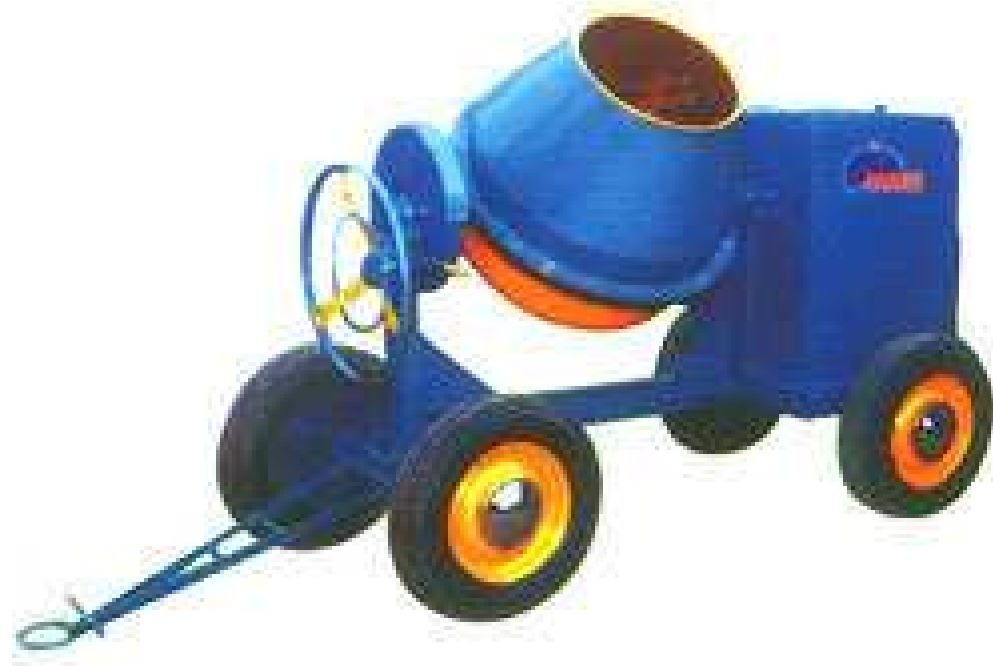
Fig. 7/5 Cft concrete mixer (3/4 bag capacity)
