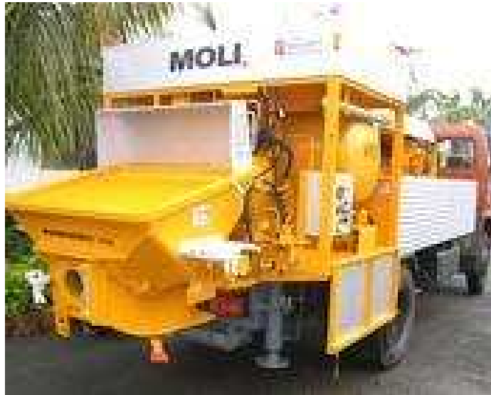
Fig.2 Truck Mounted Concrete Pumps
