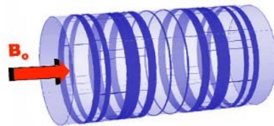
Rather than a single large/continuous winding, 6-10 large and small solenoidal bands are typically placed to create a more uniform central field with minimized fringe.
