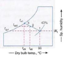
Dry bulb temperature and dew point temperature of air leaving the air washer
