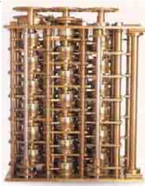
This mathematical machine called difference engine, assembled in 1832, used 2,000 levers, cams and gears.
