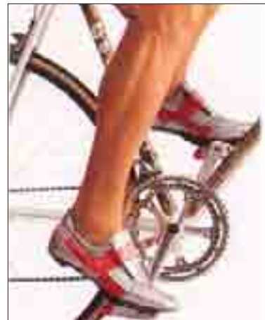
In bicycle gears are used to transmit motion. Mechanical advantage can be changed by changing gears.
