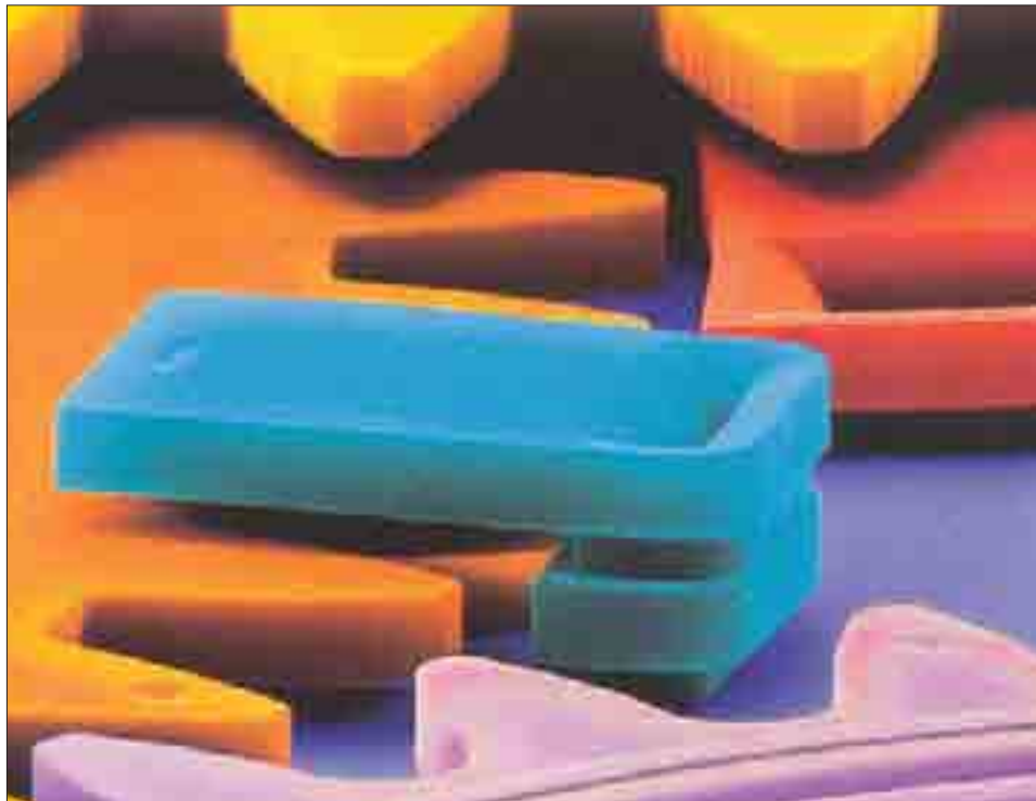
This is a close-up photo (magnified 200 times) of a micromotor's gear cogs. Micromotors have been developed for use in space missions and microsurgery.
