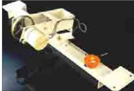
Belt slip indicator is used to indicate that the belt is slipping.
