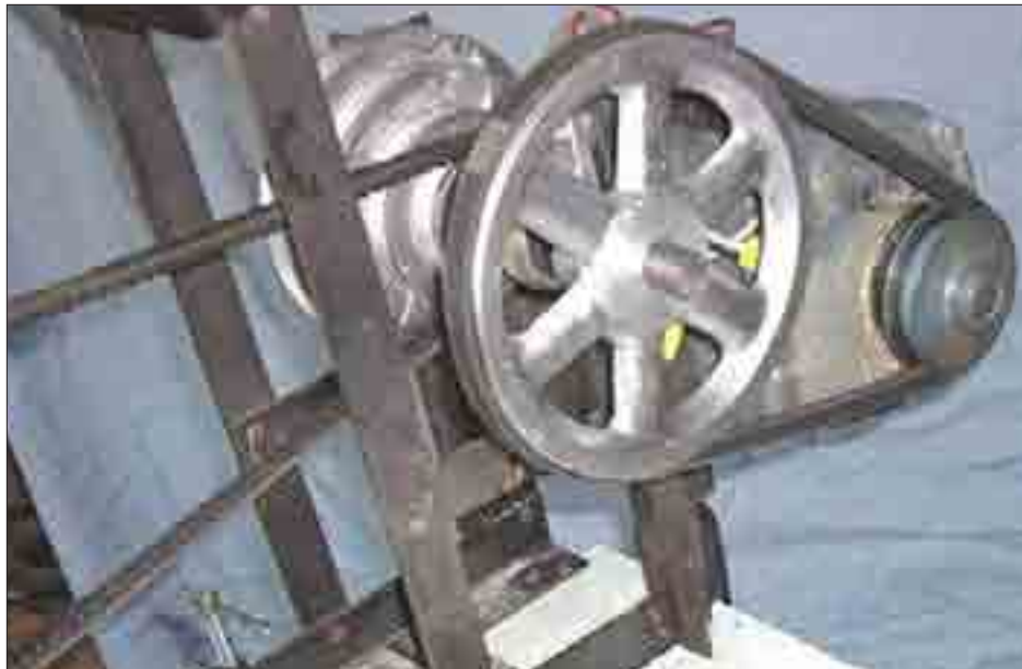
Belt drive on a lathe
