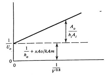
Figure 12-16 A Wilson plot to determine the individual heat-transfer coefficients of a condenser.
