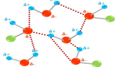
Hydrogen bonding between alcohols and water molecules
