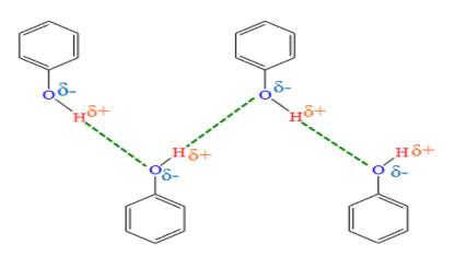
Representations of intermolecular hydrogen bonding in phenol
