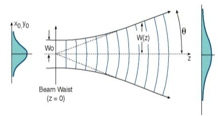
The laser beam is a single-phase Gaussian beam (TEM<sub>00</sub>) that depends on the size of the spot at the waist( $W_0$ ), the spot size at the distance from the waist (W) can be written as follows
