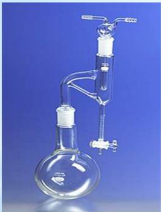
Clevenger Apparatus (Oil heavier than Water)
