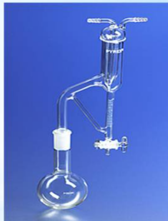
Clevenger Apparatus (Oil lighter than water)
