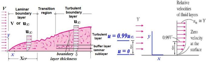
divides the flow over a plate into two regions: the *boundary layer region*, in which the *viscous effects and the velocity changes* are *significant*, and the *inviscid flow region*, in which the *frictional effects are negligible* and the velocity remains essentially constant.
