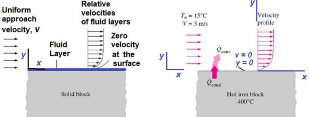
When a fluid is forced to flow over a solid surface, it is observed that the fluid in motion comes to a complete stop at the surface and assumes a zero velocity relative to the surface. That is, the fluid layer in direct contact with a solid surface "sticks" to the surface and there is *no slip*. In fluid flow, this phenomenon is known as the *no-slip condition*, and it is due to the viscosity of the fluid.
