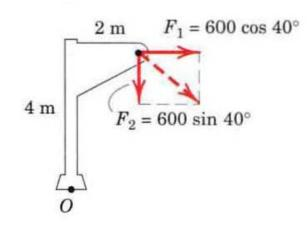
Replace the force by its rectangular components at A
