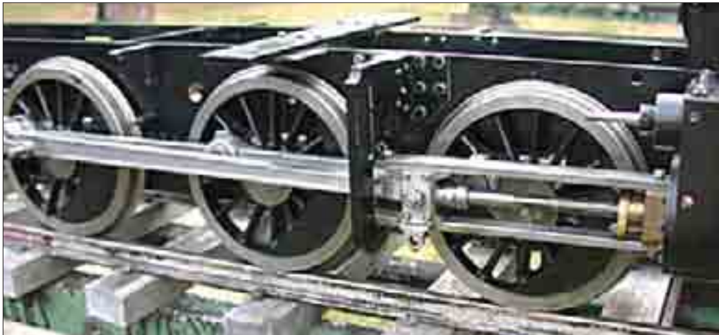
Steel tyres of a locomotive.
