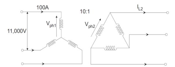
Phase voltage on the primary side,  $V_{ph1} = \frac{11,000}{\sqrt{3}} = 6.35kV$ Secondary side phase voltage,  $V_{ph2} = \frac{6.35}{10} = 0.635kV$ Secondary side line voltage = Secondary side phase voltage
