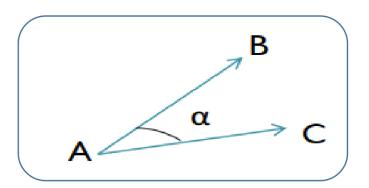
Horizontal angle is the angle between two intersected vertical planes, measured in horizontal plane. They are used to determine bearings and directions in Control surveys.
