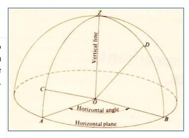
Vertical angle is the angle measured on vertical plane from zenith point to required point. Such as the angel between vertical line and line OD
