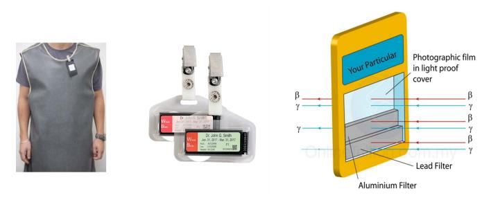
**Thermoluminescent Dosimeters** (TLDs) (مقياس جرعات التالق الحراري): are devices used to measure and record ionizing radiation exposure. They are widely used in various industries, including healthcare, nuclear power, and radiography. TLDs offer several advantages over other dosimetry methods, and here are the key points to understand about them:
