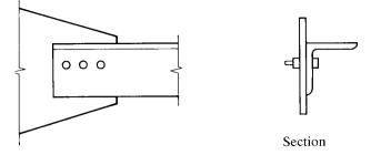
suggests that shear lag be accounted for by using a reduced, or effective, net area. Because shear lag affects both bolted and welded connections, the effective net area concept applies to both types of connections.
