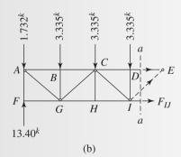
Member *IJ* is the bottom chord member with the largest force. For the free body shown in Figure 3.36b,
