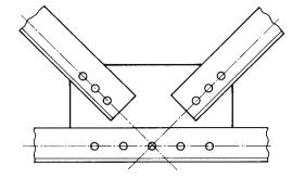
The fact that chord members are continuous and joints are bolted or welded would seem to invalidate the usual assumption that the truss is pin-connected. Joint rigidity does introduce some bending moment into the members, but it is usually small and considered to be a secondary effect. The usual practice is to ignore it. Bending caused by loads directly applied to members between the joints, however, must be taken into account. We consider this condition in Chapter 6, "Beam–Columns."
