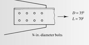
**LRFD** The factored load is **SOLUTION**  $P_u = 1.2D + 1.6L = 1.2(35) + 1.6(70) = 154$  kips Required  $A_g = \frac{P_u}{\phi_i F_y} = \frac{154}{0.90(36)} = 4.75$  in.<sup>2</sup>
