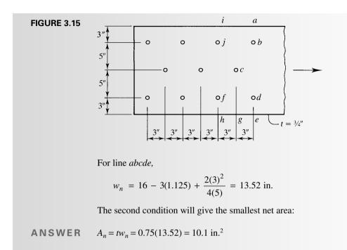
Equation 3.2 can be used directly when staggered holes are present. In the computation of the net area for line *abcde* in Example 3.6,
