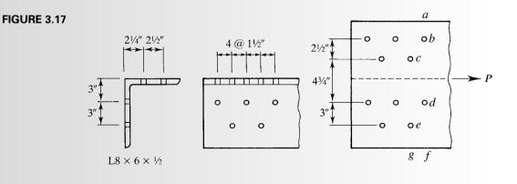
of 5.413 in.<sup>2</sup> should be multiplied by <sup>10</sup>/<sub>9</sub> to obtain a net area that can be compared with those lines that resist the full load. Use  $A_n = 5.413(^{10}/_{9}) = 6.014$  in.<sup>2</sup> For line *abcdeg*,
