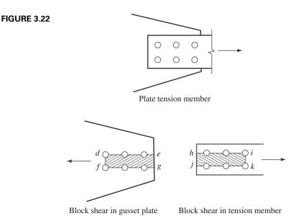
stress, so the nominal strength in shear is  $0.6F_uA_{nv}$  and the nominal strength in tension is  $F_uA_{nt}$ ,
