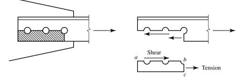
For the case illustrated, the shaded block would tend to fail by shear along the longitudinal section ab and by tension on the transverse section bc.
