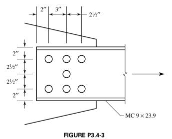
**3.4-4** A992 steel is used for the tension member shown in Figure P3.4-4. The bolts are  $\frac{3}{4}$  inch in diameter. The connection is to a  $\frac{3}{-}$ -in.-thick gusset plate.
