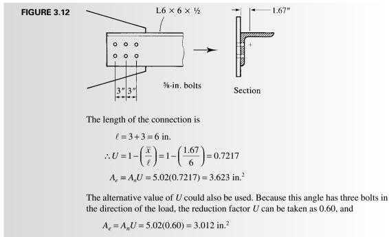
Either U value is acceptable, and the Specification permits the larger one to be used. However, the value obtained from Equation 3.1 is more accurate. The alternative values of U can be useful during preliminary design, when actual section properties and connection details are not known.
