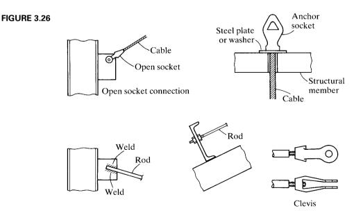
The effective cross-sectional area in the threaded portion of a rod is called the *stress area* and is a function of the unthreaded diameter and the number of threads per inch. The ratio of stress area to nominal area varies but has a lower bound of approximately 0.75. The nominal tensile strength of the threaded rod can therefore be written as
