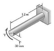
The solid shaft shown is made of a mild steel that is assumed to be elastoplastic with G = 77.2 GPa and  $\tau_{\rm Y} = 145$  MPa. Determine the angle of twist caused by the application of a torque of magnitude (a)  $T = 600 \text{ N} \cdot \text{m}$ , (b)  $T = 1000 \text{ N} \cdot \text{m}$ .
