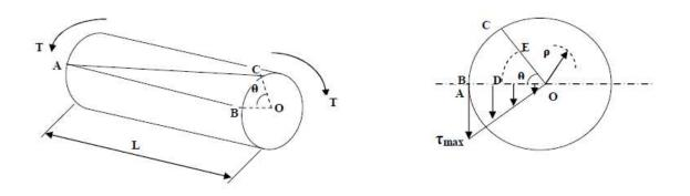
If the torque (T) is applied at the free end of the shaft, the fiber (AB) on outside surface will be twisted into (AC) as the shaft is twisted through the angle ( $\phi$ ). Consider any internal fiber located a radial distance (R) from the axis (Centre of the shaft), the radius will also rotate through angle ( $\phi$ ) causing total shearing deformation ( $\tau$ ) equal to arc length (DE).
