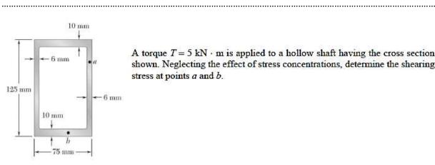
A torque  $T = 5 \text{ kN} \cdot \text{m}$  is applied to a hollow shaft having the cross section shown. Neglecting the effect of stress concentrations, determine the shearing stress at points a and b.
