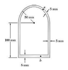
A 5.6 kN m torque is applied to a hollow shaft having the cross section shown. Neglecting the effect of stress concentrations, determine the shearing stress at points a and b.
