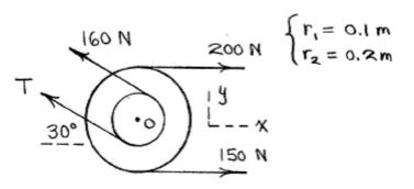
+)  $M_0 = 0$ : 200(0.2) - 150(0.2) - 160(0.1) + (0.1)T = 0 T = 60 N  $R_x = \Sigma F_x = 200 + 150 - (160 + 60) \cos 30^\circ = 159.5 N$   $R_y = \Sigma F_y = (160 + 30) \sin 30^\circ = 110 N$   $R = \sqrt{R_x^2 + R_y^2} = \frac{193.7 N}{193.7 N}$  $\Theta = \tan^{-1} (\frac{R_y}{R_x}) = 34.6^\circ$
