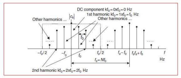
For convenience, we compute the spectrum over the range from 0 to  $f_s$  Hz with nonnegative indices, that is,
