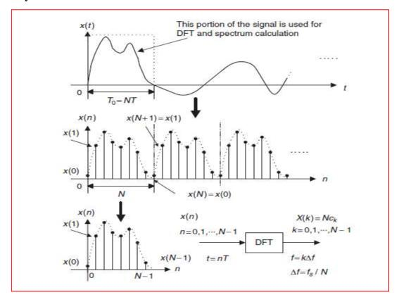
First, we assume that the process acquires data samples from digitizing the interested continuous signal for duration of T seconds. Next, we assume that a
