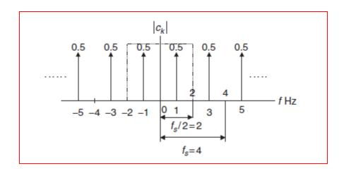
As we know, the spectrum in the range of -2 to 2 Hz presents the information of the sinusoid with a frequency of 1 Hz and a peak value of  $2|c_1| = 1$  which is converted from two sides to one side by doubling the spectral value. Note that we do not double the direct-current (DC) component, that is,  $c_0$ .
