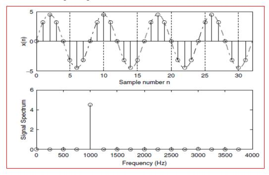
The algorithm transforming the time domain signal samples to the frequency domain components is known as the discrete Fourier transform, or DFT.
