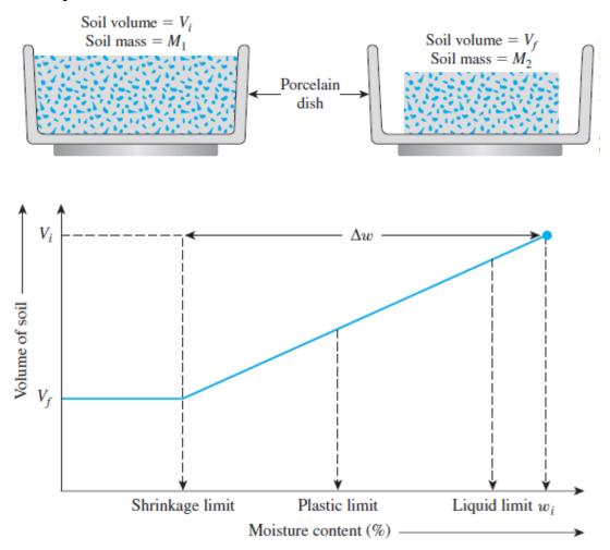
the shrinkage limit can be determined as
