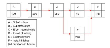
**Figure 1** The construction plan for each house.
