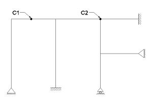
r > C+3, the frame is stable & indeterminate  $5^{th}$  degree.
