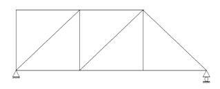
The truss is stable &determinate
