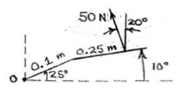
$$G \ge M_0 = 50 \cos 20^\circ [0.1 \cos 25^\circ + 0.25 \cos 10^\circ] + 50 \sin 20^\circ [0.1 \sin 25^\circ + 0.25 \sin 10^\circ] = 17.29 \text{ N·m}$$
