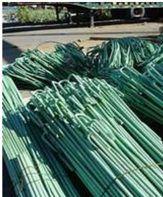
Pic.(40): steel reinforcing protected with epoxy
