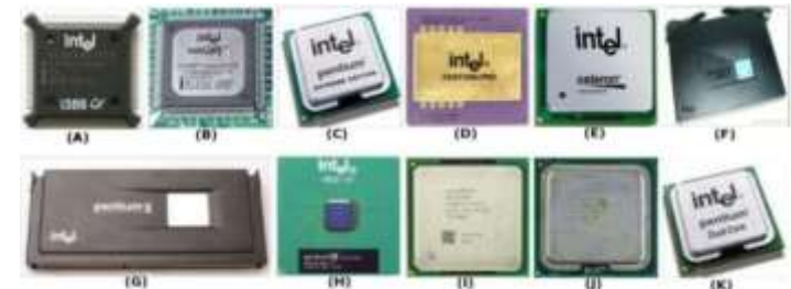
Figure 1.6: 32-bit Microprocessors: (A) 80386, (B) 80486, (C) Pentium (80586), (D) Pentium Pro, (E) Celeron, (F) Pentium II Xeon, (G) Pentium II, (H) Pentium III, (I) Pentium IV, (J) Pentium D, and (K) Pentium Dual-
