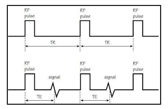
Fig.(2): A basic pulse sequence.
