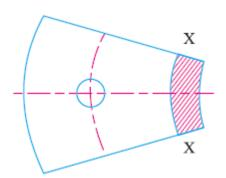
e =Pitch circle radius – (Radius of bolt hole + Thickness of cylinder wall)
