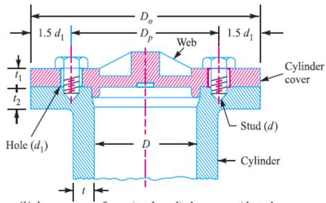
(b) Arrangement of securing the cylinder cover with studs.
