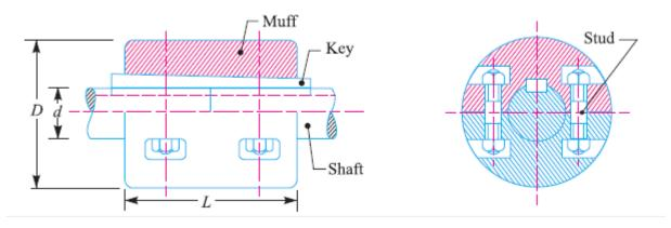
In the clamp or compression coupling, the power is transmitted from one shaft to the other by means of key and the friction between the muff and shaft. In designing this type of coupling, the following procedure may be adopted.
