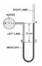
Case (1): Pressures at B = Pressures at C
