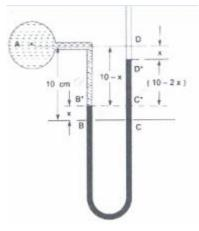
If the value of  $P_A$  is becomes is 9810 N/m<sup>2</sup>, i.e is less than the 12360.6 N/m<sup>2</sup>, hence mercury in left limb will rise, this rise of mercury in the left limb is equal to the fall of mercury in the right limb, because the volume of mercury remains same .
