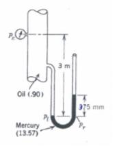
The pressures over the datum  $P_L$  -  $P_r$  in two sides are equal :
