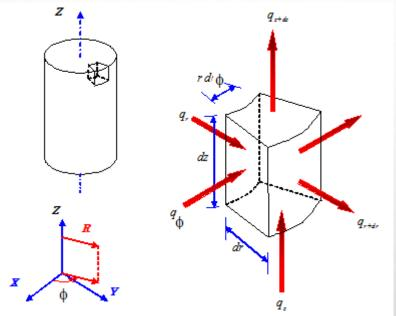
$\frac{1}{r}\frac{\partial}{\partial r}\left(r\frac{\partial T}{\partial r}\right) + \frac{1}{r^2}\frac{\partial}{\partial \phi}\left(\frac{\partial T}{\partial \phi}\right) + \frac{\partial}{\partial z}\left(\frac{\partial T}{\partial z}\right) + \frac{\dot{g}}{k} = \frac{1}{\alpha}\frac{\partial T}{\partial \tau}$
