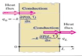
Next, We consider a heat supply into the body at the rate of  $|\dot{q}_L = 200 W / m^2$  through the boundary surface at x=L, as illustrated in Fig. 2.9. The energy balance at the surface at x=L.  $\begin{cases}
